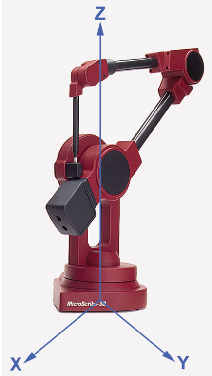
FIGURE 10 - The default start-up orientation of the MicroScribe.
