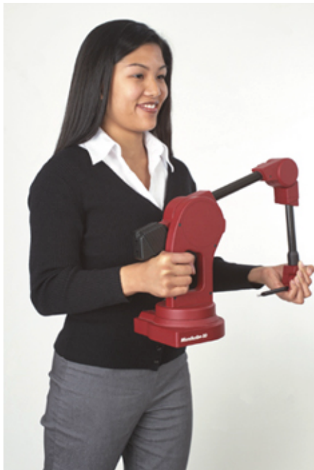
Figure 6 - The proper way to carry a MicroScribe.
